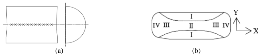
Figure 5 Hardness testing positions across the rolling direction of the specimens (a) Initial specimen, and (b) Forged specimen.
