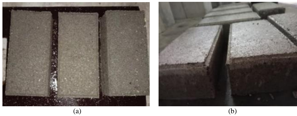
Figure 1 Visual comparison of paving blocks (a) Normal variation and (b) Addition of \text{TiO}_2\text{-SiO}_2 composite variation
