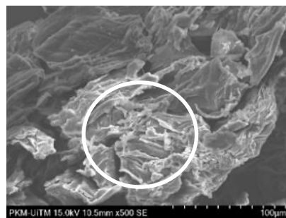
Figure 7 1340μm before extraction with finer and rough threadlike fibers
