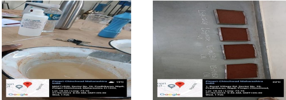
Figure 7 Chitosan biopolymer solution and Lateritic Soil Treated with Varying Chitosan Biopolymer Concentrations
