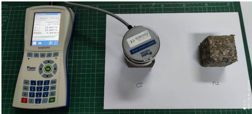
Figure 7 Thermal conductivity test of the geopolymer mortar
