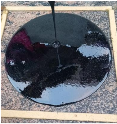
Figure 2 Mould used for the preparation of epoxy with boron carbide composites
