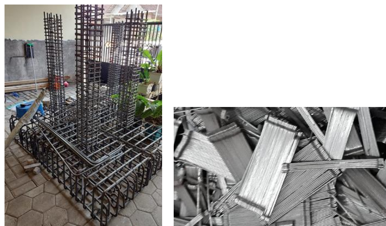
Figure 2 Column reinforcement cage and steel fiber used with aspect ratio l/d = 80
