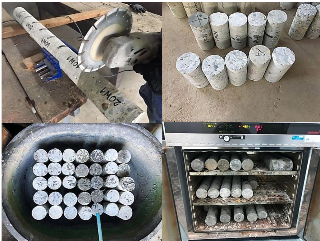
Figure 5 Laboratory prepared of concrete coring cylinder specimens for water absorption testing
