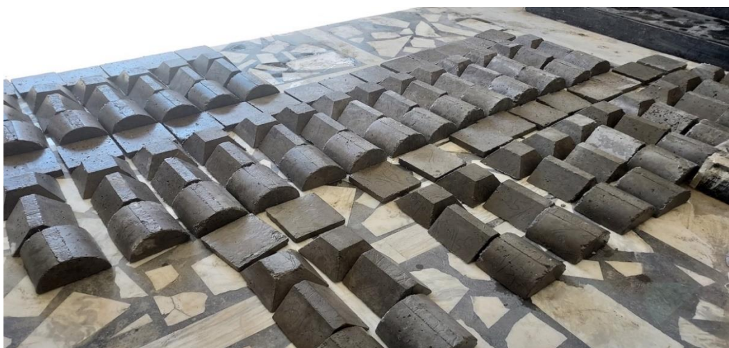
Figure 3 Prepared sample of foundation models for the load test
