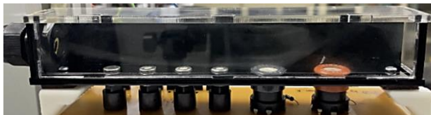
Figure 7 Smoke flow exhibits laminar flow pattern.
