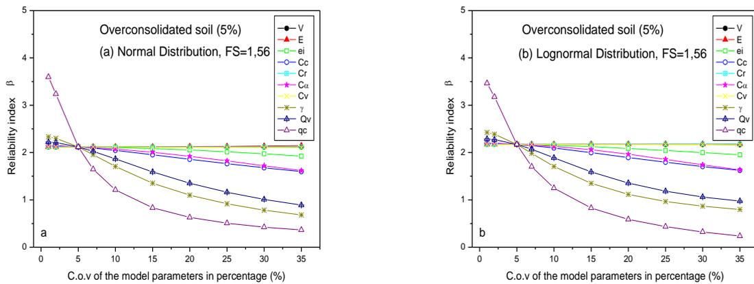
**Figure 3** Variation of reliability index with coefficient of variation (C.o.v) of settlement parameters - overconsolidated soil. (a) Normal distribution, (b) Lognormal distribution
