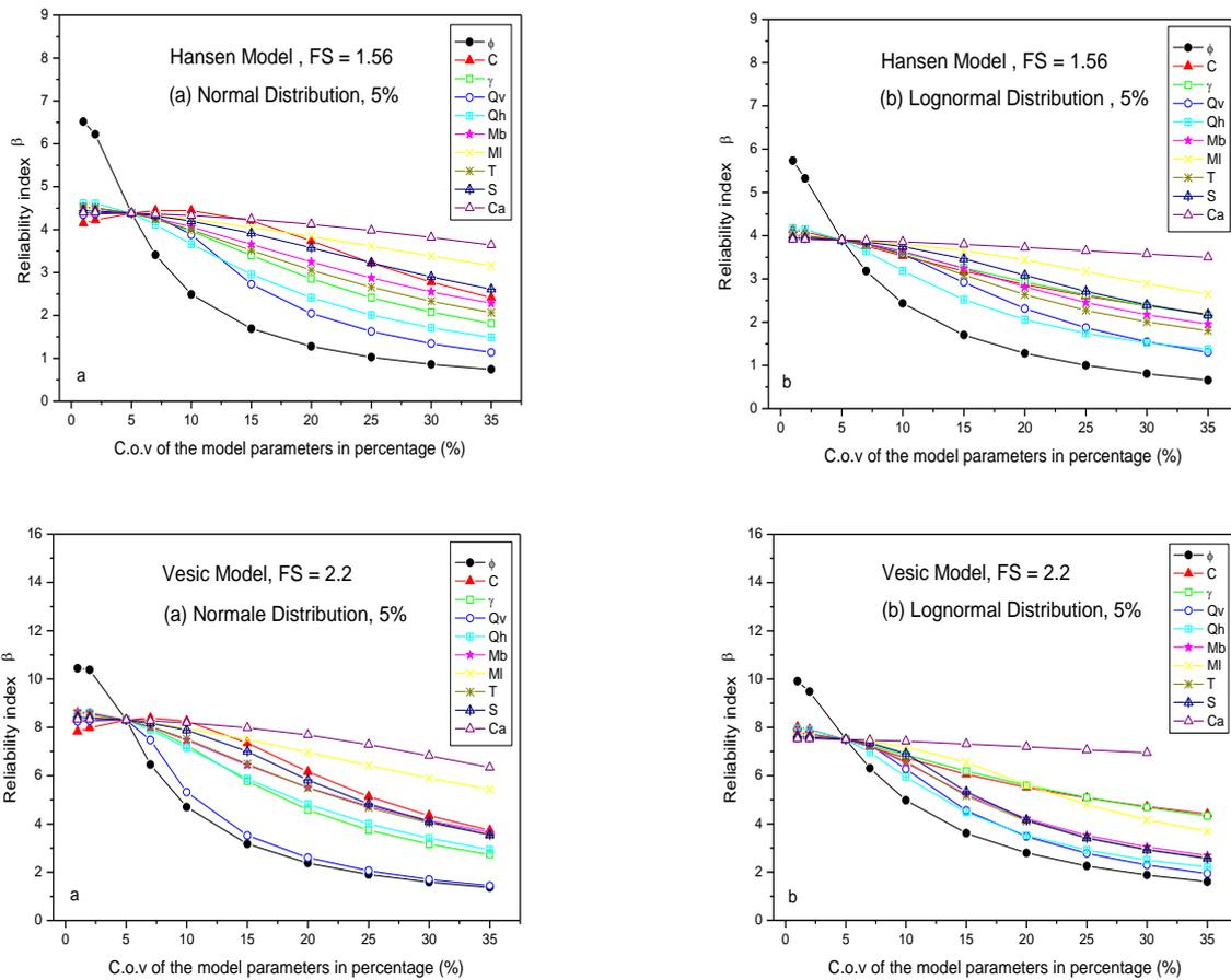
**Figure 2** Variation of the reliability index with the coefficient of variation (C.o.v) of the capacity parameters of shallow foundations. (a) Normal distribution, (b) Lognormal distribution.
