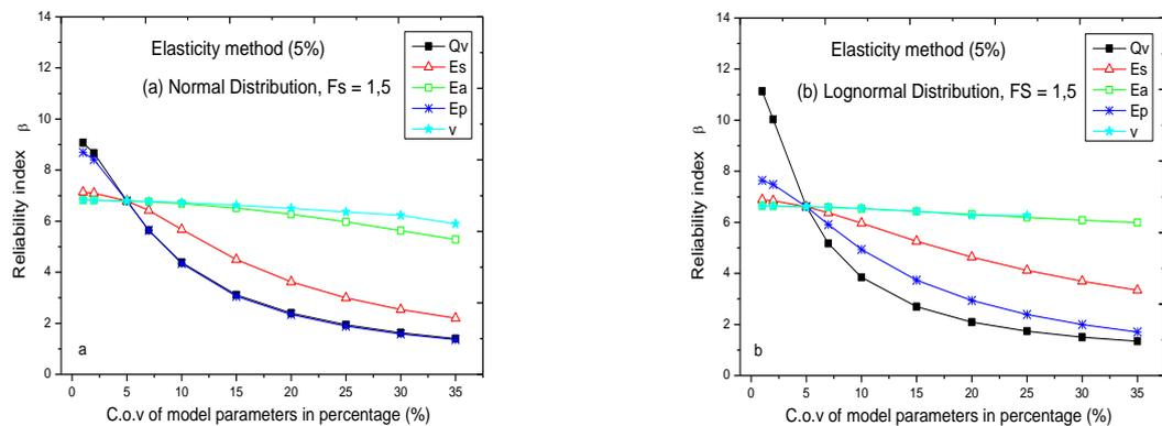
**Figure 9** Variation of reliability index with coefficient of variation of settlement parameters for an isolated pile. (a) Normal distribution, (b) Lognormal distribution.
