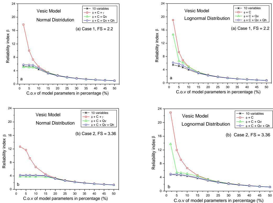
Figure 7 Reduction of random parameters - Vesic model. (a) Case 1, (b) Case 2.
