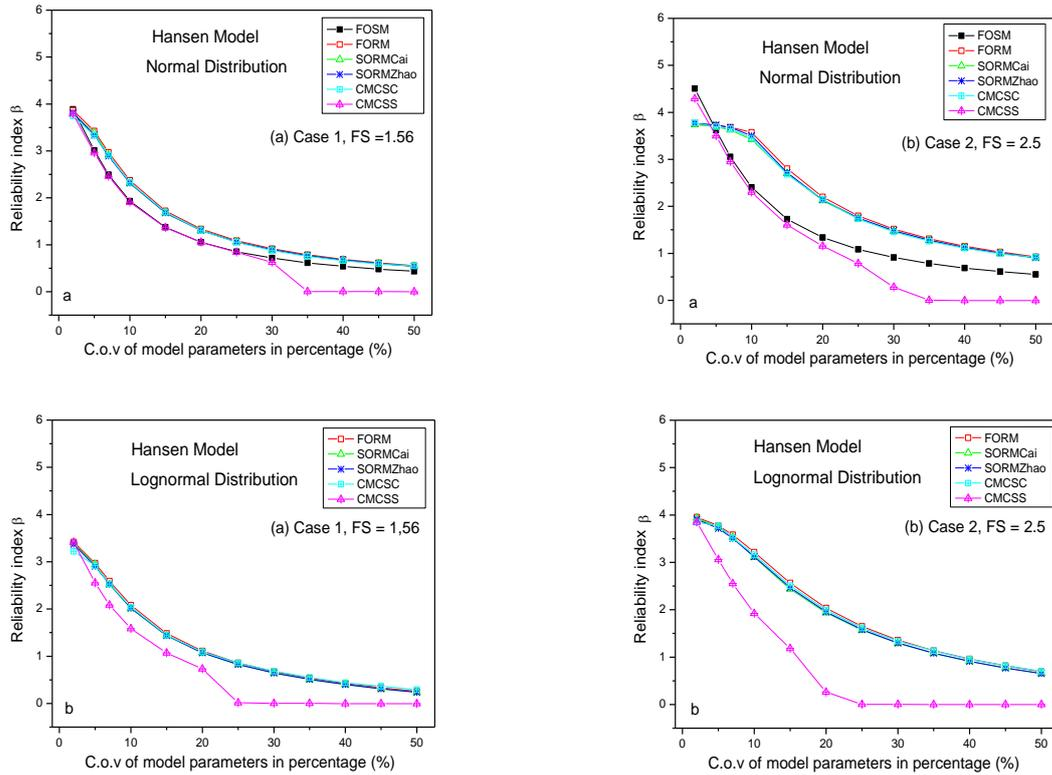
**Figure 4** Comparison of reliability indices calculated with FOSM, FORM, SORM, and MCS - Hansen model. (a) Case 1, (b) Case 2.
