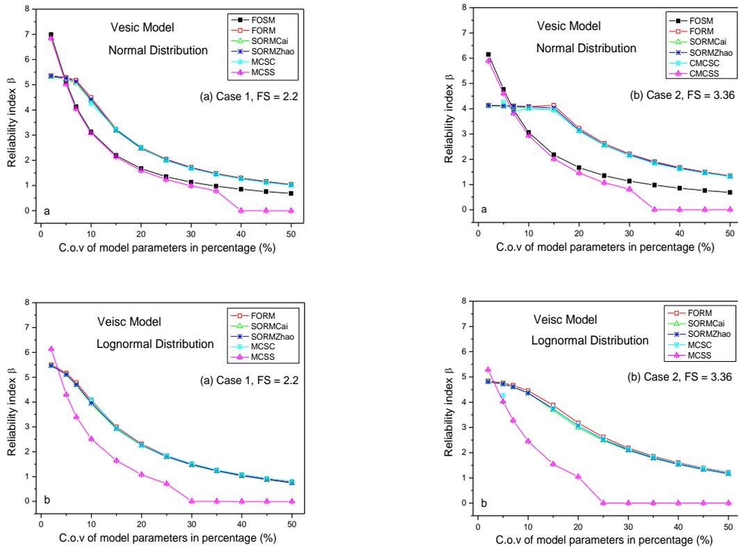
**Figure 5** Comparison of reliability indices calculated with FOSM, FORM, SORM, and MCS - Vesic model. (a) Case 1, (b) Case 2.
