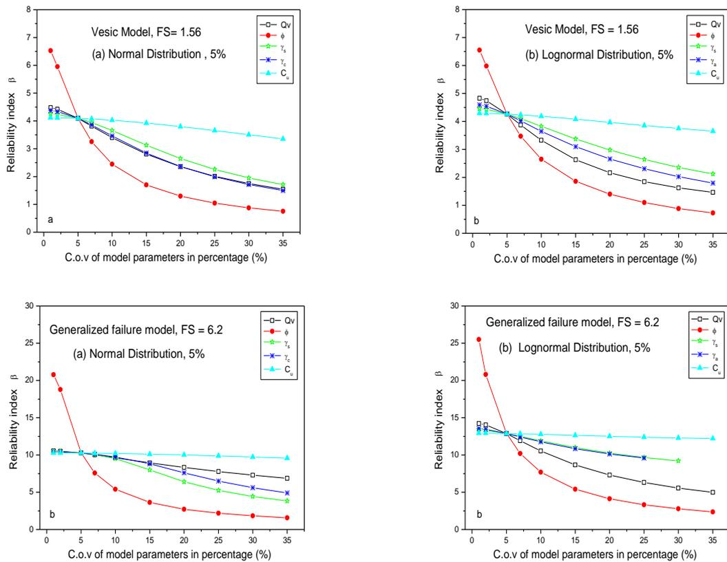
**Figure 8** Variation of the reliability index with the coefficient of variation (C.o.v) of the parameters for the bearing capacity of an isolated pile. (a) Normal distribution, (b) Lognormal distribution.
