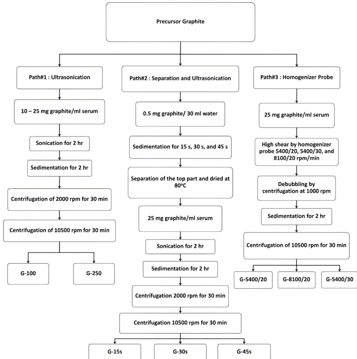
Figure 1 The schemes of graphite exfoliation in three proposed paths to yield various exfoliated graphite samples are proposed.
