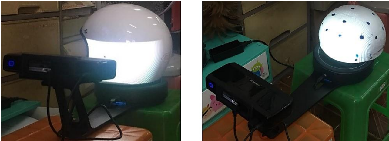
Figure 4 3D-Scan technique to obtain a file of the helmet piece
