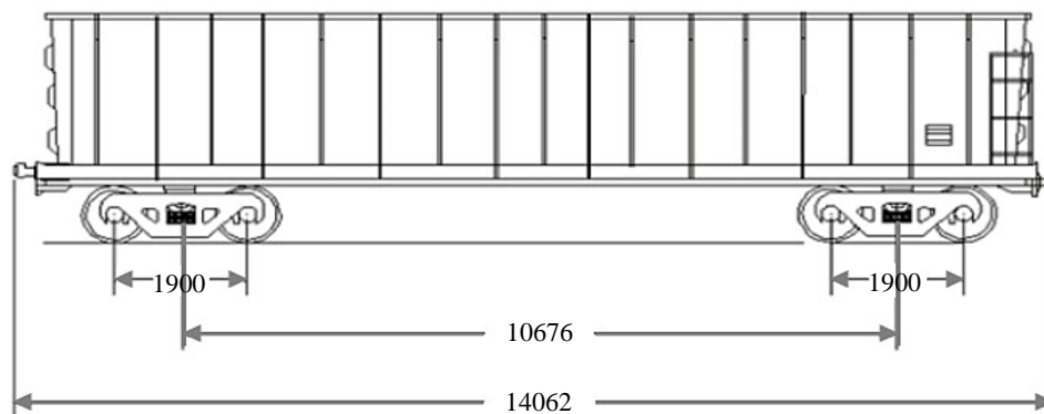
Figure 3 Distance between two bogies ( L_b ) in the coal wagon of Babaranjang freight train [4]
