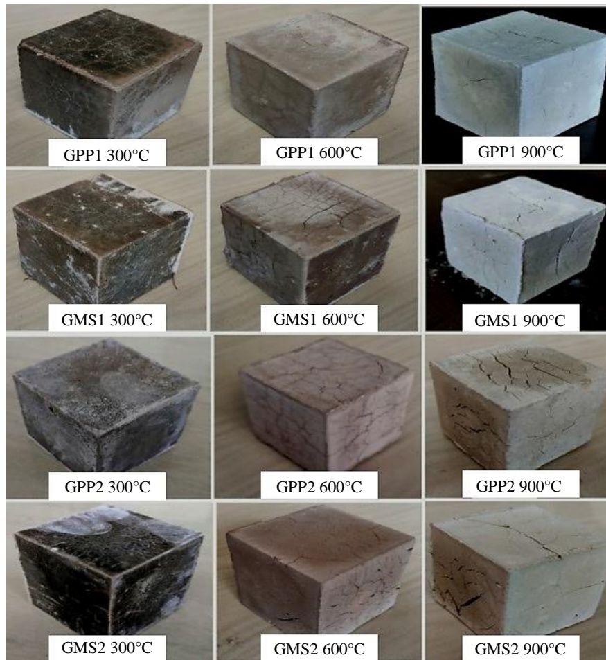
Figure 10 Surface image of fiber reinforced AAC paste samples
