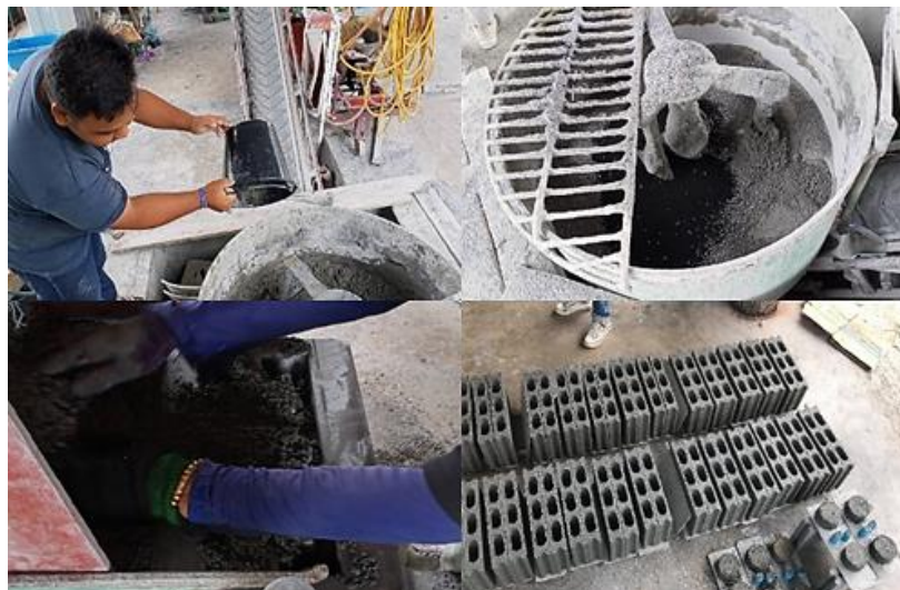
Figure 3 Concrete block manufacturing process in the factory
