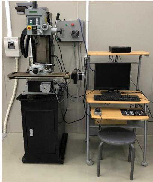
**Figure 4** A general view of CNC milling machine used in each experiment
