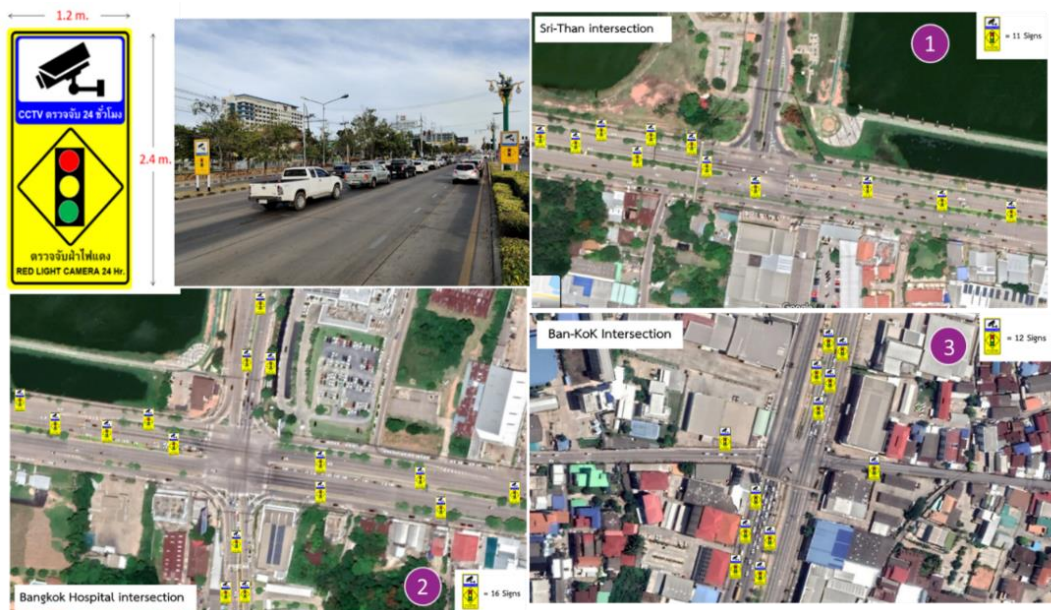
Figure 2 Examples of the installation and the points of the sign installation at the 3 intersections under the red-light camera project
