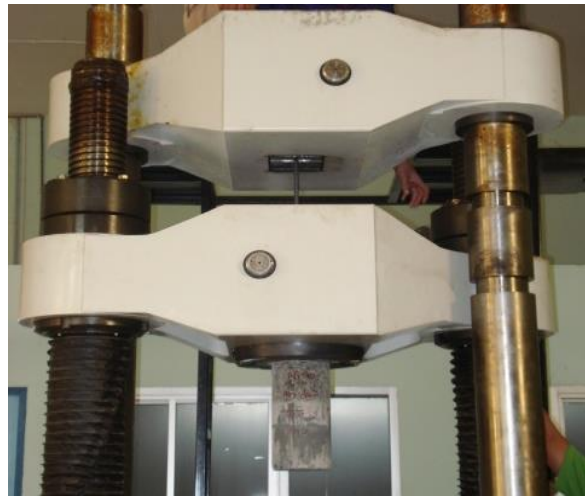
Figure 4 Configuration of pull-out test using UTM
