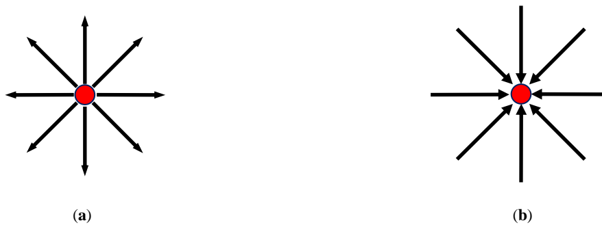
Figure 4 Divergence of a vector field: (a) positive divergence and (b) negative divergence
