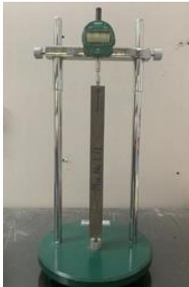
**Figure 2** Drying shrinkage test setup
