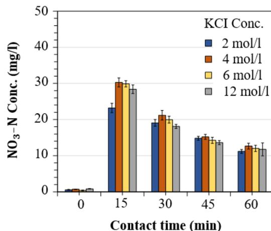
**Figure 5** The changes of nitrate-nitrogen yield in various KCl concentrations during air plasma treatment at various treatment times.
