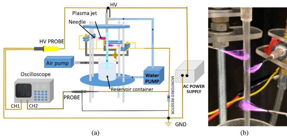
**Figure 1** (a) A schematic drawing of the plasma model and the experimental setup, and (b) Image of MBR water stream being treated by multi-air plasma jets.
