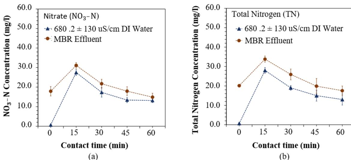
**Figure 3** (a) Nitrate-nitrogen concentration, and (b) Total nitrogen concentration in MBR effluent and EC-adjusted DI water at various treatment times.
