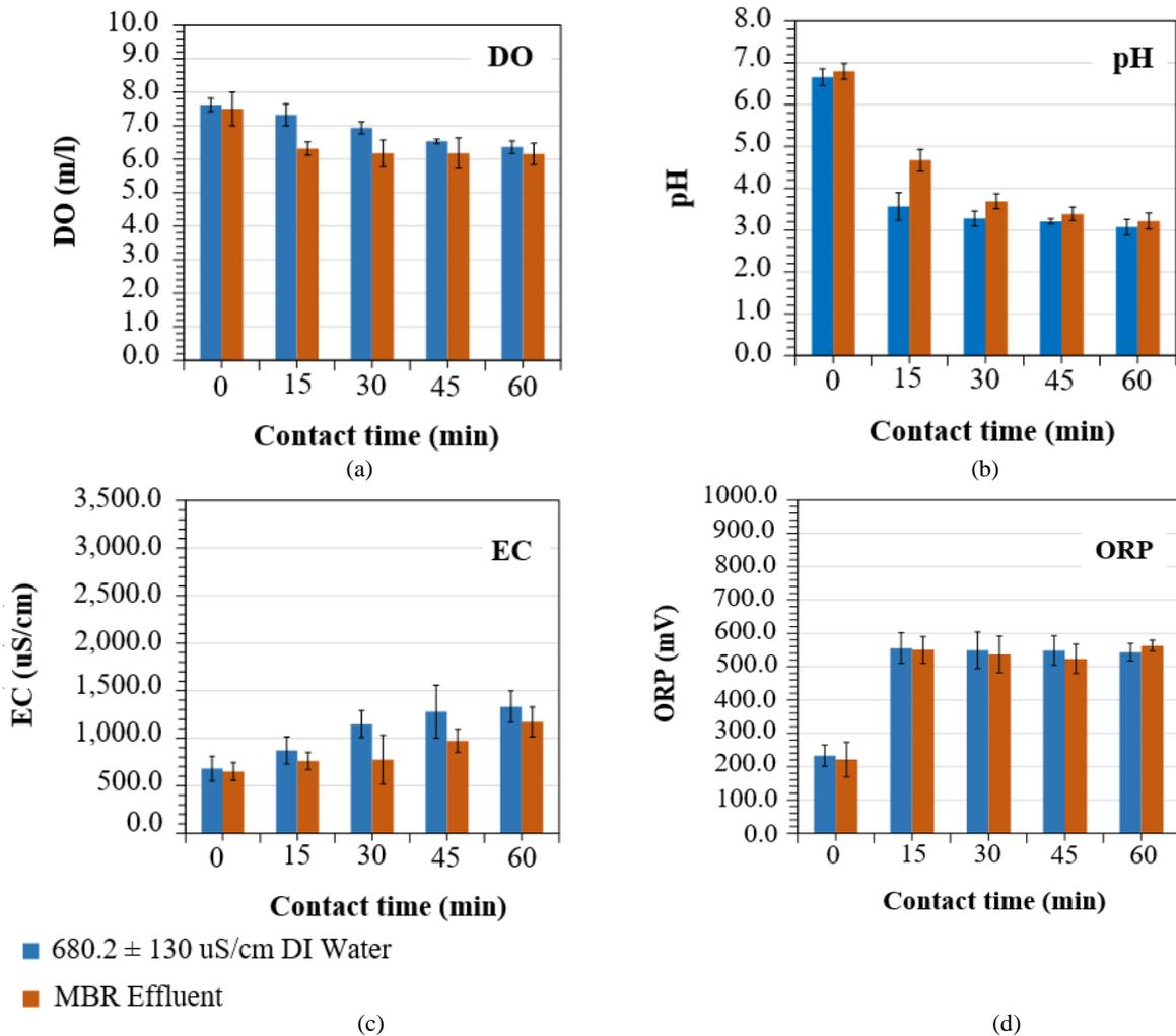
**Figure 4** (a) DO, (b) pH, (c) EC, and (d) ORP of liquid media samples after air plasma treatment at various treatment times.
