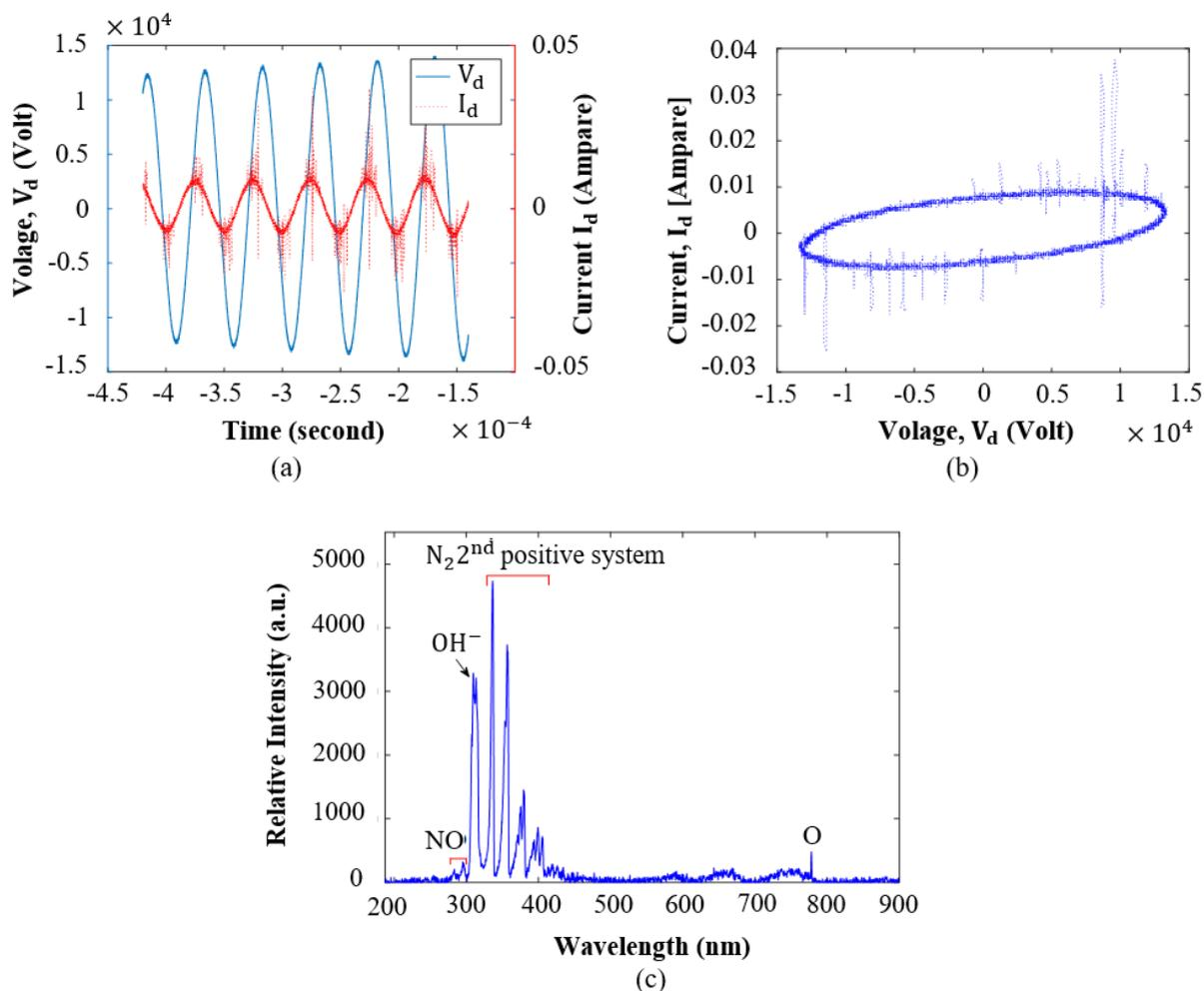
**Figure 2** (a) Electrical characteristics of voltage and current waveforms, (b) The voltage and current plot over one period, and (c) Optical emission spectra of air plasma jets.
