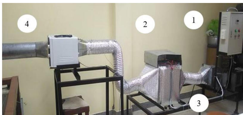
Figure 1 Microwave-assisted hot air dryer apparatus consisted of 1) controller 2) heater 3) blower 4) drying chamber
