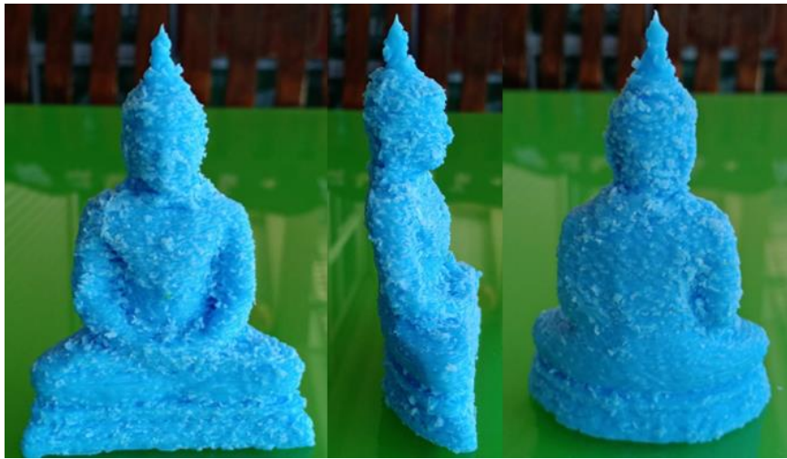
Figure 9 The 3D-buddha image model made of injection-grade wax
