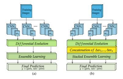
Figure 1 Illustration of the ensemble convolutional neural network architectures using differential evolution algorithms with mutation strategy. (a) Ensemble-CNN method and (b) Stacked Ensemble-CNN method.
