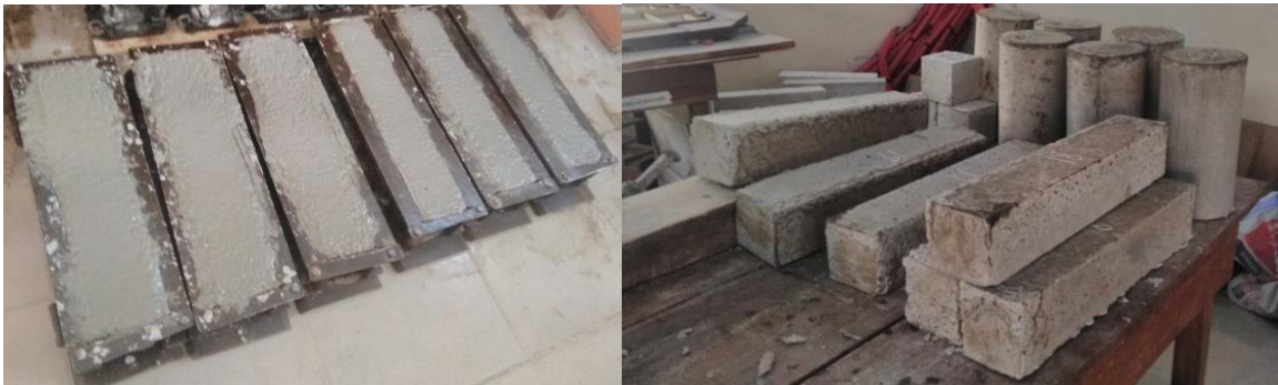
Figure 4 Concrete beam and cylinder samples
