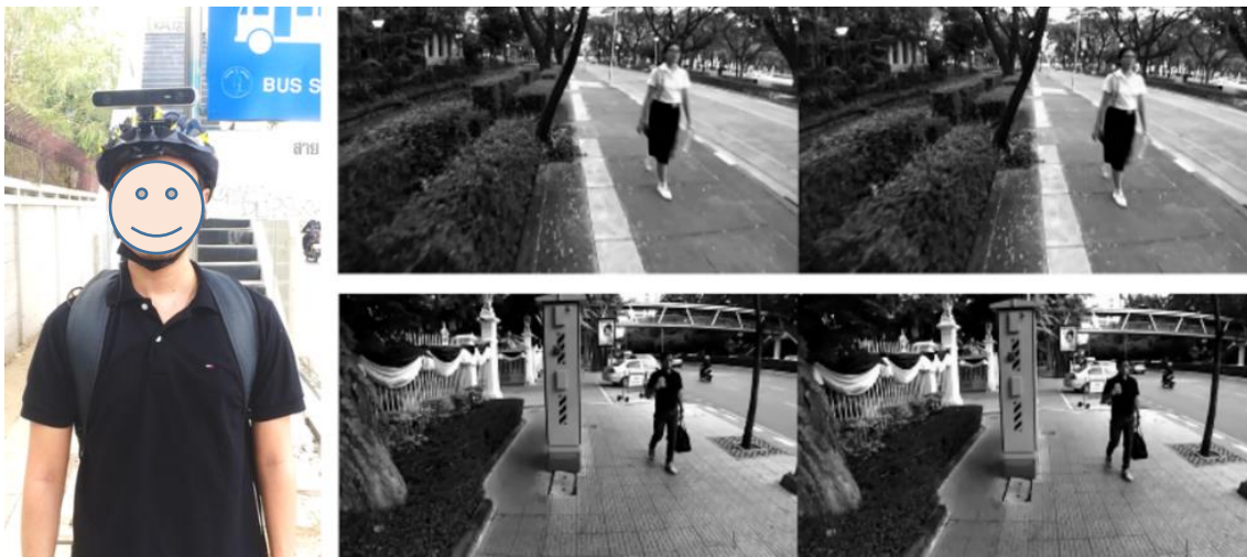
Figure 12 Stereo camera mounted on data collector head (left), the example of stereo image for data acquisition process (right)
