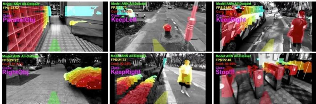
Figure 10 The example resulting interface of our obstacle classification and navigation system
