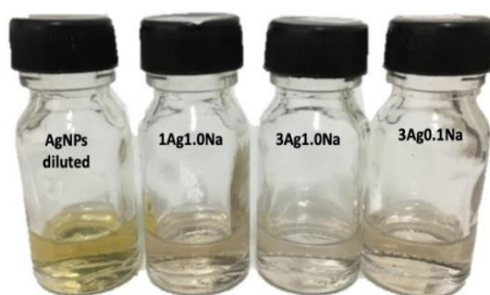
Figure 5 The left-most bottle shows the yellow color of AgNPs before reaction. The faded samples (the other three samples) are seen after the reaction with H_2O_2 solution
