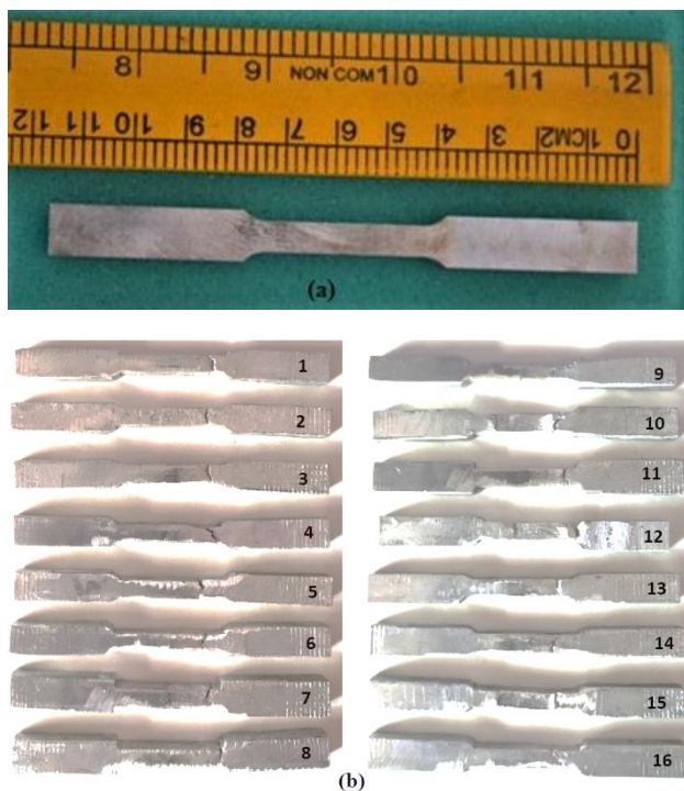
Figure 6 Photographic images of tensile test specimens (a) before fracture and (b) after fracture
