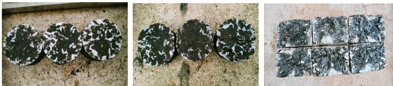
Figure 5 Samples before (a) and after (b and c) the ITS test
