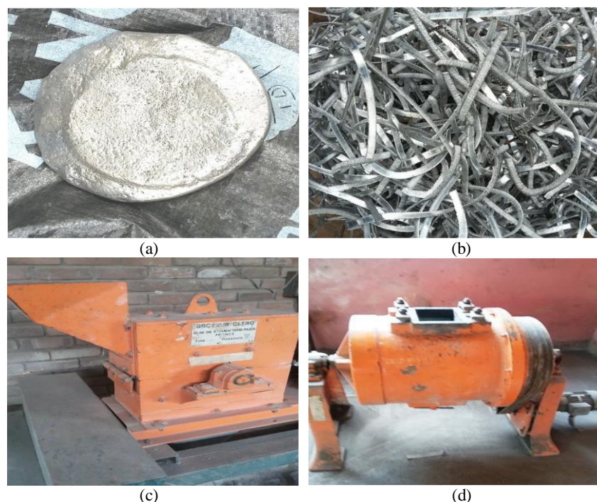
Figure 3 Procedure for recycling of aluminium can scraps: (a) cast ingot powder; (b) chips from cast ingot; (c) crusher and (d) ball mill
