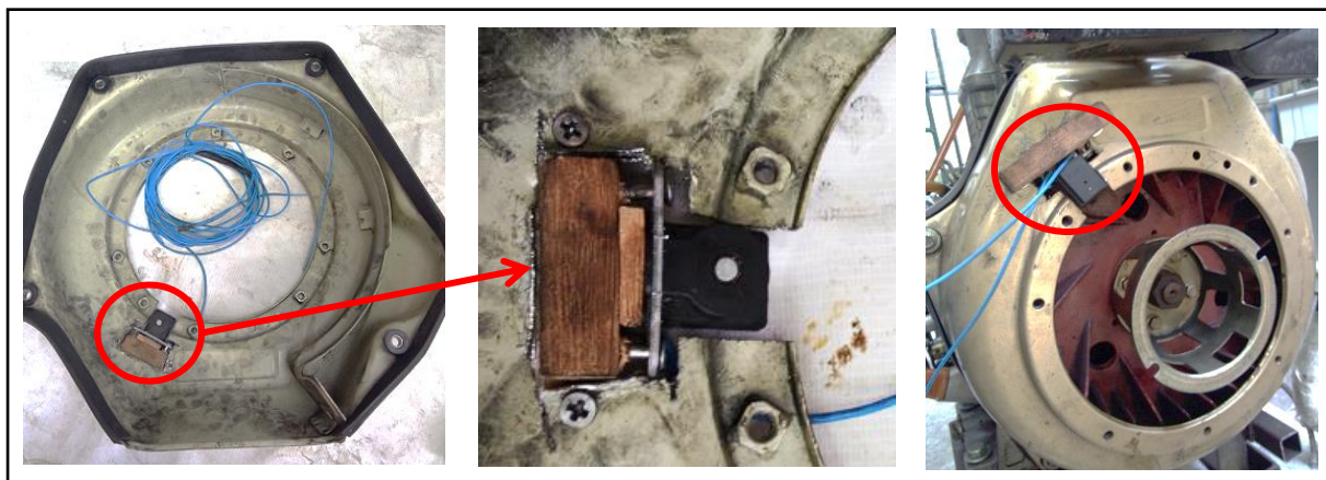
Figure 6 An inductive type sensor mounted on a fan casing to detect fan blades
