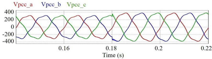
Figure 20 The PCC voltage under voltage rise
