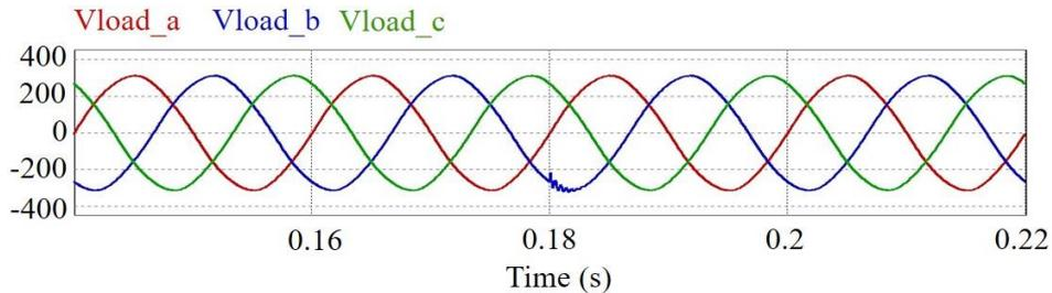
Figure 15 The load voltage after compensation for an unbalanced fault
