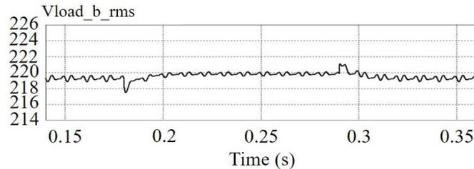
**Figure 28** The dynamic response of the conventional compensator for an unbalanced fault (SLGF)
