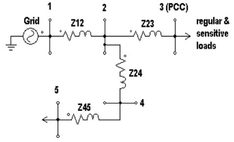
**Figure 5** A typical electric network under study [7]
