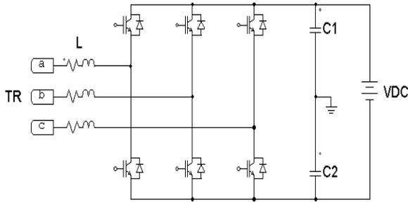
**Figure 1** The three-phase four-wire VC-VSI power circuit
