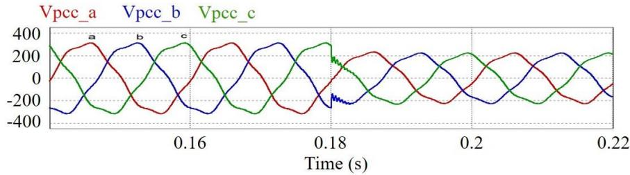
**Figure 8** The PCC voltage under a balanced fault at bus 4
