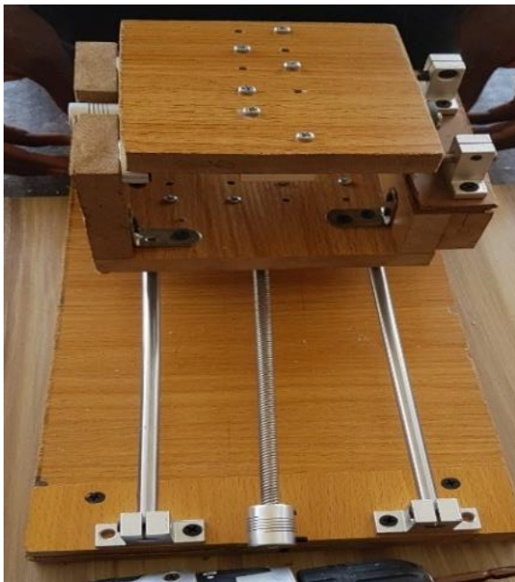
Figure 10 Attaching the Z-axis assembly to the Y-axis
