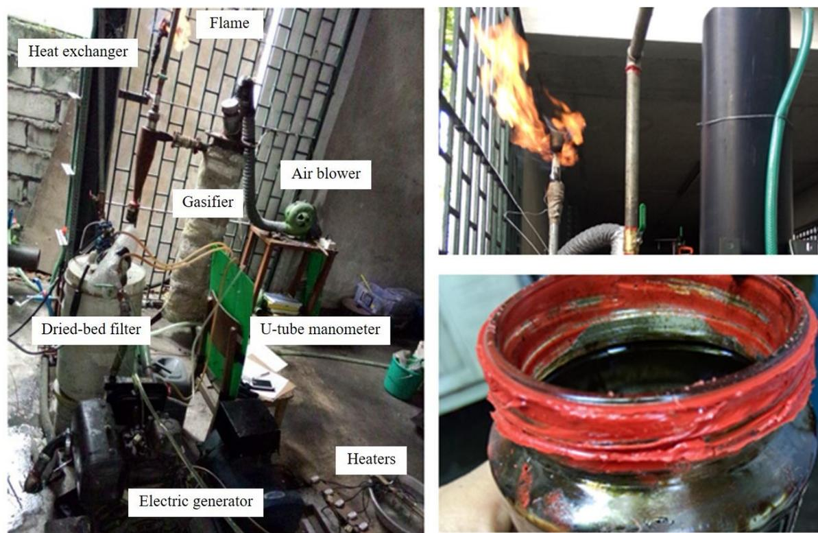
**Figure 8** Gasifier-generator unit (left), producer gas flame (upper right), and tar (lower right)
