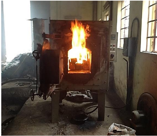
Figure 1 Samples being subjected to a fire test inside an electric-fired furnace
