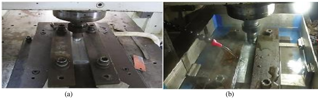
Figure 1 Experimental setup for (a) conventional FSW and (b) UFSW [14]
