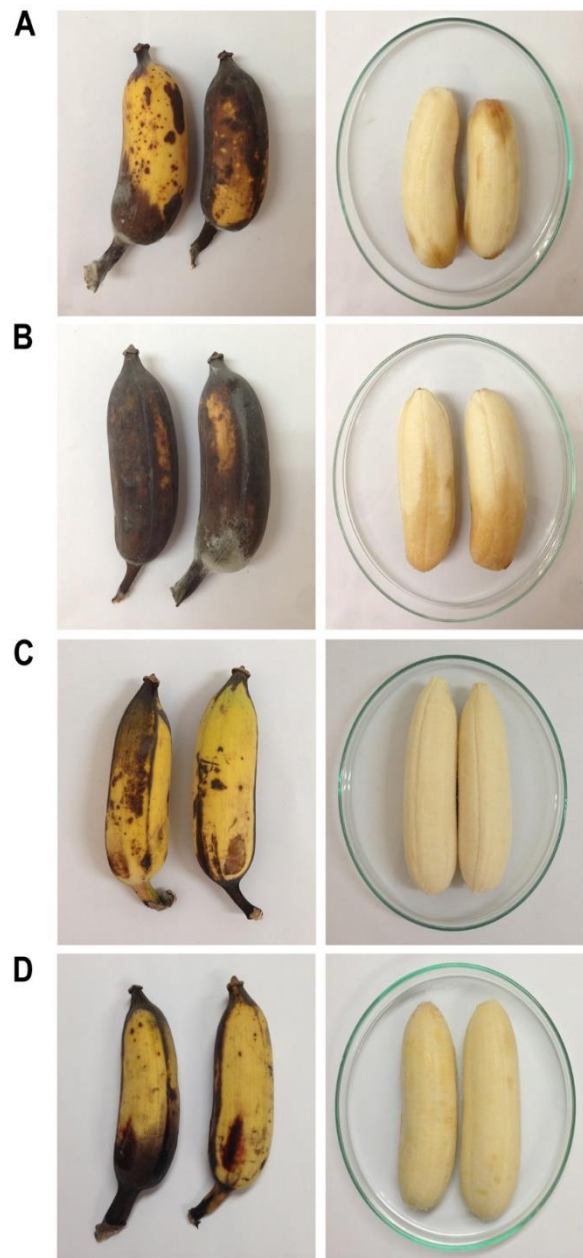
Figure 7 Physical appearance of bananas packaged for 12 days in a bag made of PLA blend /5 wt % RHA (A); PLA blend /10 wt% RHA (B); PLA blend /20 wt% RHA (C) and PLA blend /20 wt% RHA for 14 days (D), all films were stretched at a 150 rpm screw speed
