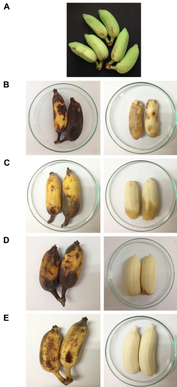
Figure 6 Physical appearance of bananas as received (A) and after storing for 8 days without packaging (B) with a conventional LLDPE bag (C); PLA blend film, stretched at 150 rpm screw speed (D); PLA blend /20 wt% RHA, stretched at 150 rpm screw speed (E)
