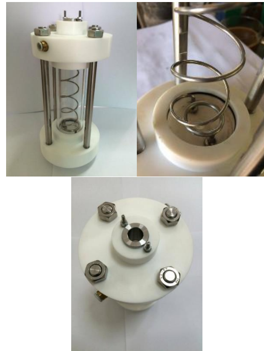
Figure 3 The prototype of the reverse vortex flow gliding arc discharge reactor
