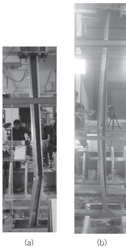
Figure: 9 Local-flexural torsional buckling of stud with tracks (a) 1800 mm column and (b) 2400 mm columns.
