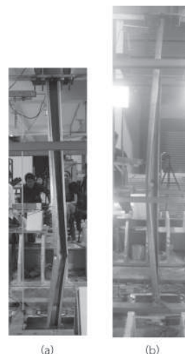
Figure: 6 Flexural torsional buckling combined with local buckling in studs (a) 1800 mm column and (b) 2400 mm column.
