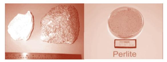
Figure 1 Perlite samples and ground perlite.
