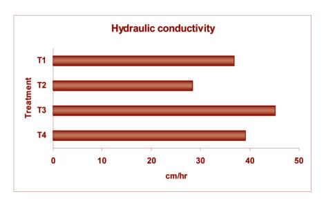
Figure 4 Hydraulic conductivity values of growth materials.
