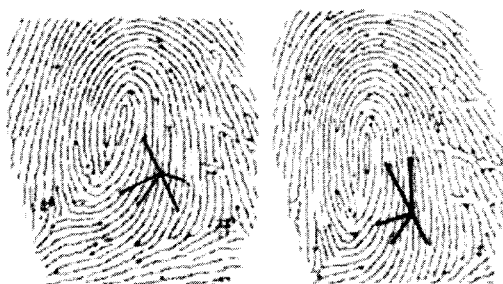
Figure 4: The example of extracted feature (minutiae) with two fingerprints.
