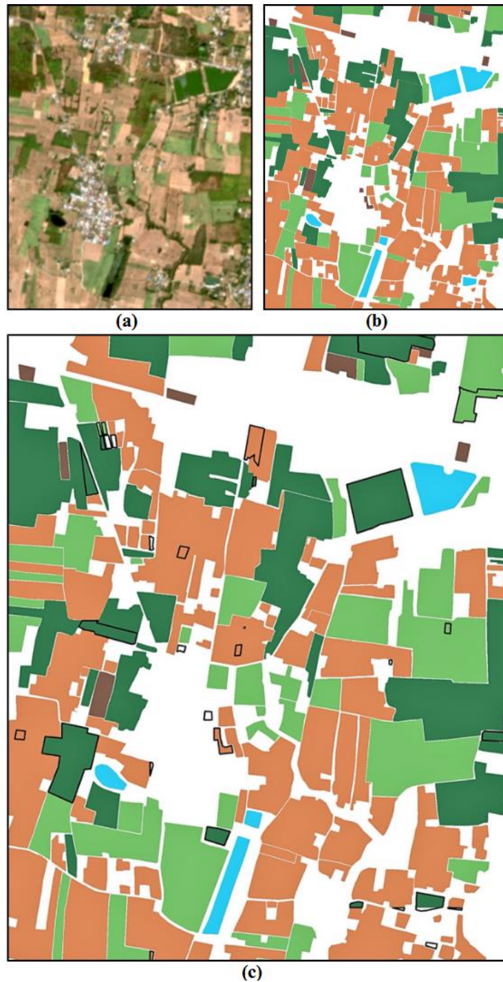
Figure 5 Comparison of the input Sentinel-2 satellite image (a), annotated segmentation (ground truth labeled) image (b), and final segmentation map (c) at a resolution of 2,088 x 2,600 pixels, derived from the training and validation datasets after reconstruction and majority color processing
