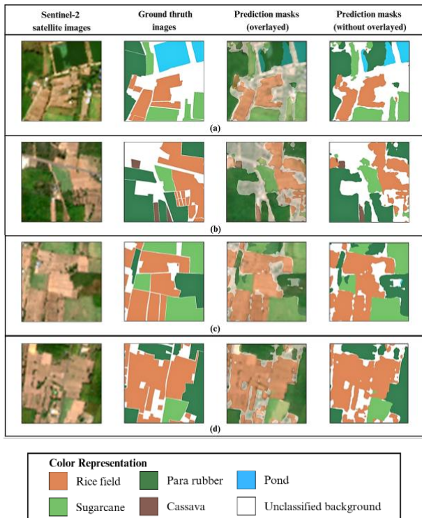
Figure 4 Inference comparison using the training and validation datasets. Panels a–d represent different patch locations. The colors highlight different classes: rice (orange), sugarcane (light green), para rubber trees (dark green), cassava (brown), and pond (blue).
