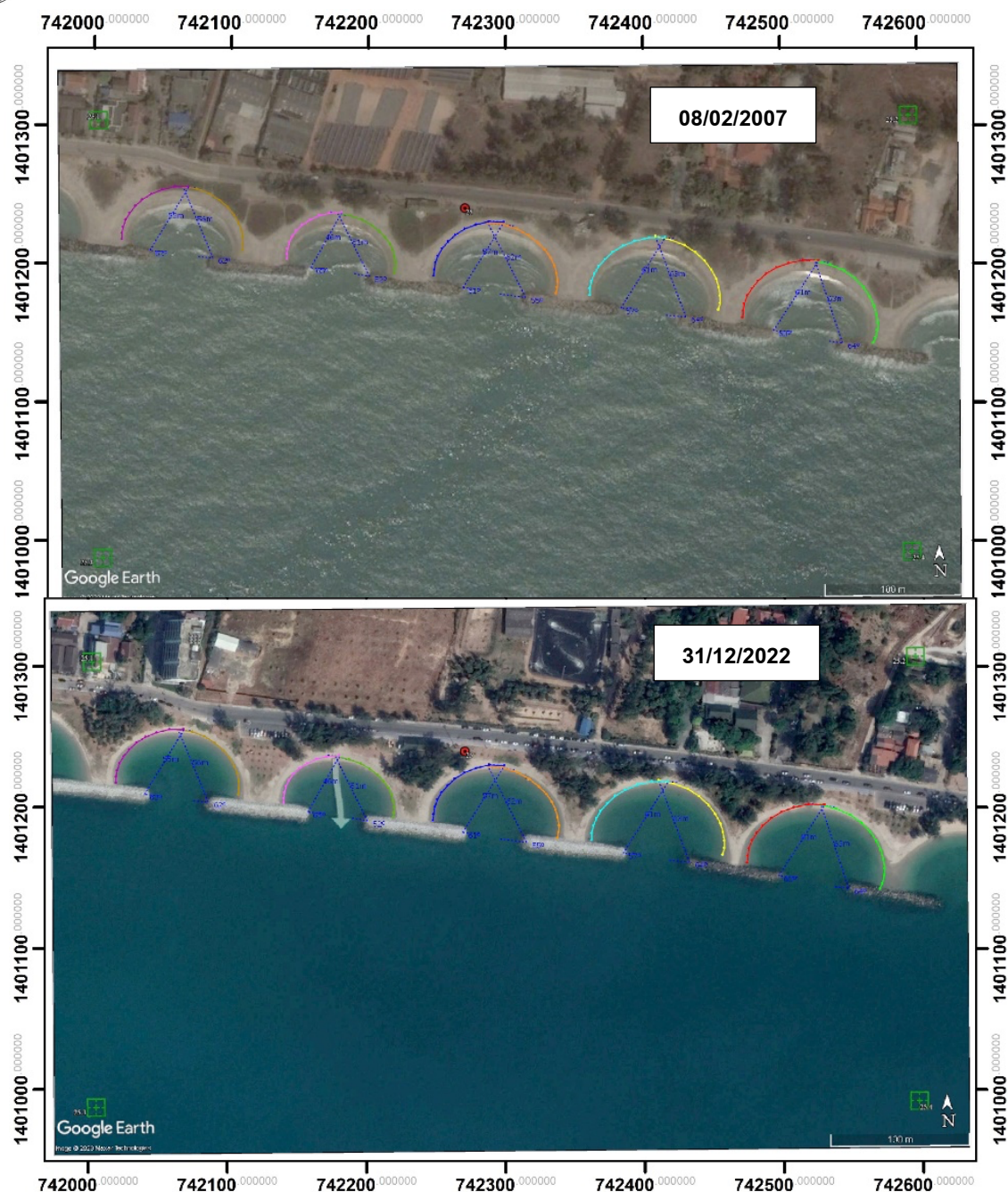
Figure 3. MEPBAY analysis of existing detached breakwaters at Saengchan Beach in Rayong province (courtesy of Google Earth) (The distinct hues of the line represent different diffraction points).
