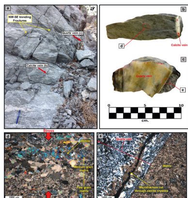
Figure 15: Outcrop characteristics in Area 3 (a) Both calcite veins and quartz veins show the dominant NW-SE trending fracture trend. (b), (c) Slab face samples of calcite veins and quartz veins with attached matrix. (d) Photomicrograph showing banding in marble is caused by combination of different crystal sizes and aligned platy minerals, mostly biotite. (e) Microfracture cutting through, with calcite crystals precipitated within a quartz vein.
