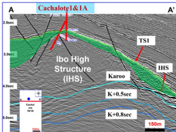
Figure 18. Cachalote 1&1A, cross-section, lower Cretaceous poroperm reservoirs distribution.
