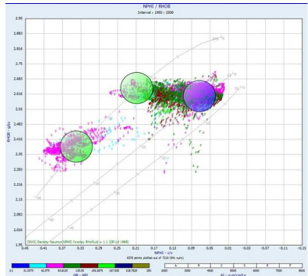
Figure 5.1. Cachalote 1&1A, compatible crossplots, apparent matrix density, cement type evaluation. The lower Cretaceous sand facies trends to dolomite whereas the upper Jurassic enhances limestone trend.
