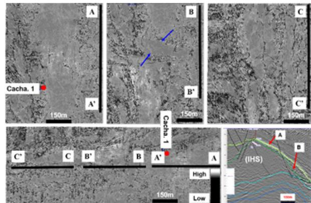
Figure 10. Cachalote 1&1A, Semblance. Structural features such normal faults: NW/SE; NNW/SSE and NNE/SSW and slump scar (blue arrows).
