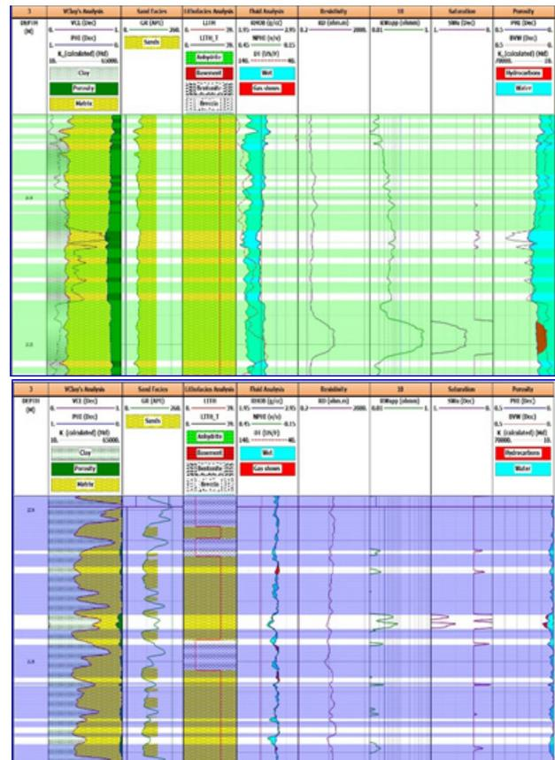
Figure 5.2. Cachalote 1&1A, apparent matrix density, cement type evaluation. Blue shadow represents lower Cretaceous and blue the upper Jurassic cement type's distribution based on the crossplots.
