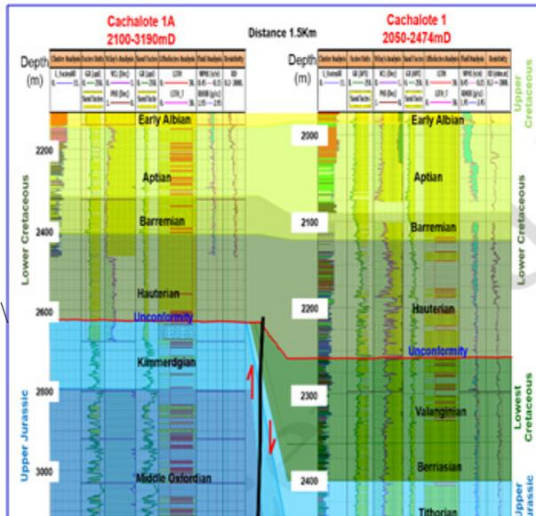
**Figure 14.** Cachalote 1&1A, chronostratigraphic correlation. Thrust fault and unconformity mark the major event within Cachalote 1&1A lithofacies.
