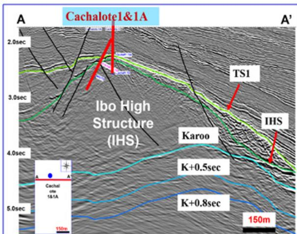
Figure 8. Cachalote 1&1A. TWT cross-section, shows the Top Sand 1 (TS1), Ibo High Structure (IHS) and Karoo horizons and Karoo +0.5sec; +0.8sec strata slices
