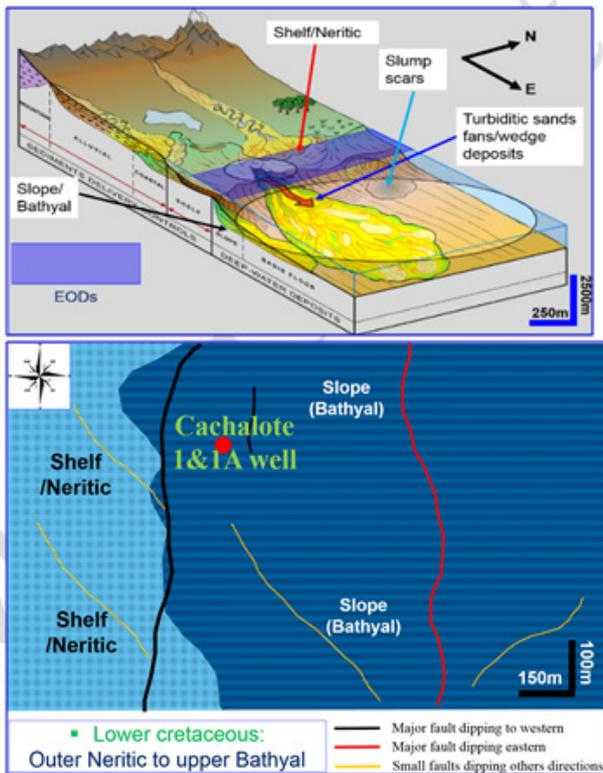
Figure 17. Cachalote 1&1A, 3D and top view of the depositional environments paleomodelling.
