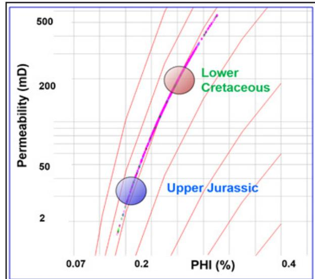
Figure 6. Cachalote 1&1A, poroperm evaluation. Lower Cretaceous shows relative good poroperm properties response than upper Jurassic.
