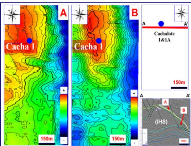
Figure 9. Cachalote 1&1A, TWT structural maps (TS1), Ibo High Structure horizons slices. The positive represents shallower and blue the deep section. Erosional clues are enhanced by contouring control.
