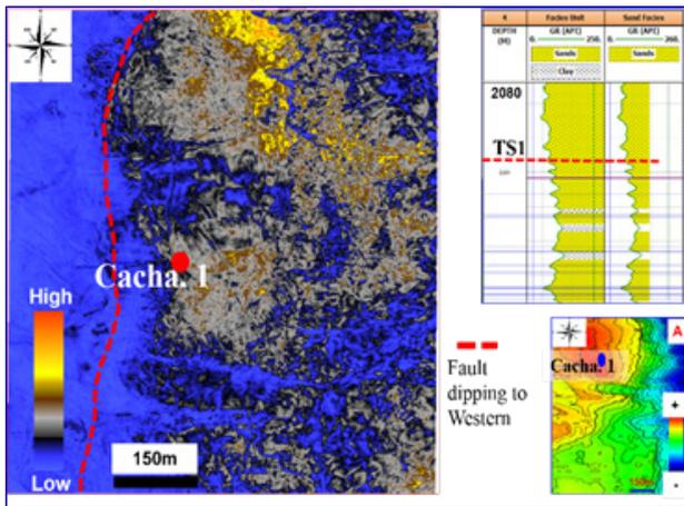
**Figure 12.** Cachalote 1&1A, SDE at 16Hz enhances channels features (black arrows) and slump scar (red arrows). Small channels trend W-E, NW-SE are potential source of the sand facies distribution.
