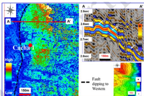
**Figure 13.** Cachalote 1&1A, SDT at 16Hz based on TS1 horizon slice. High amplitude enhances the sand thickness facies distribution.
