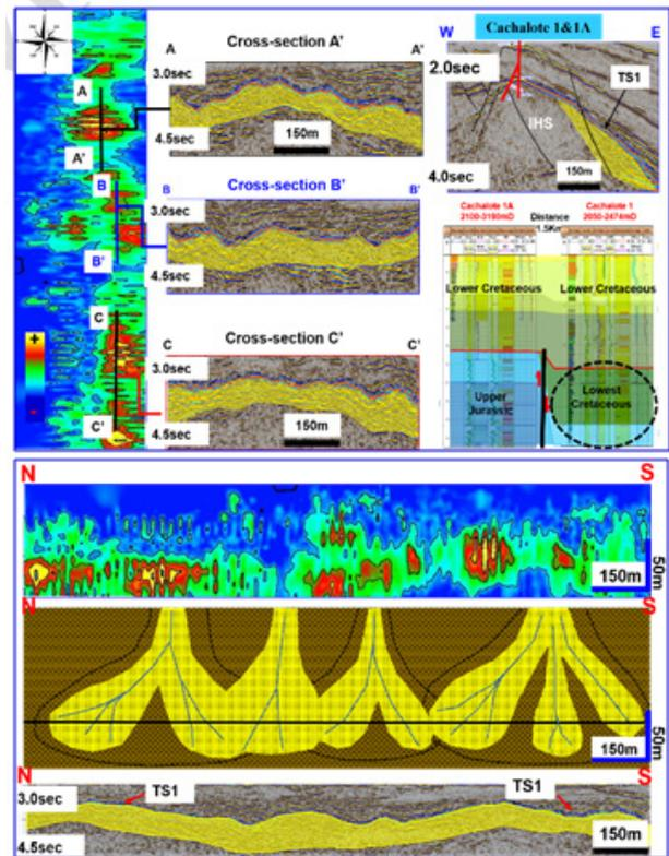
Figure 16.2. Cachalote 1&1A, Isochronal eastern and top view lower Cretaceous reservoir maps, distribution.
