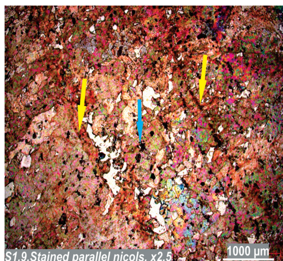
Figure 7. Thin section indicates the enclosed laminated layers (yellow arrows) showing a typical poikilotopic set of aligned calcite crystals that compose many of the speleothem textures. Also shows zones of crosscutting vuggy or dissolution porosity (turquoise arrow).
