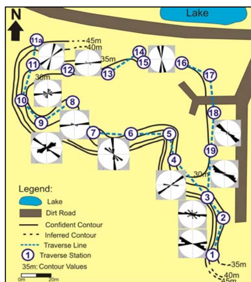
Figure 6: The stereographic plots of fractures orientations for the whole outcrop. Main orientations are N-S, NW-SE and E-W.
