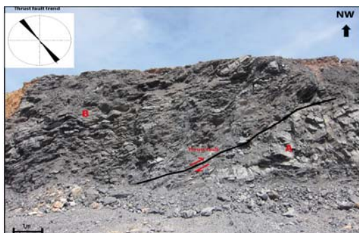
Figure 5. Photo of thrust fault and shear zone in the subarea-2 at outcrop A12. (A) Medium to thick bed limestone (unit 3), (B) Thin to medium bed limestone (unit 4)
