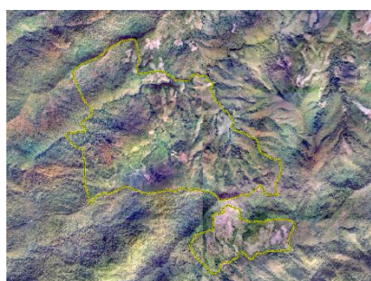
Figure 11 Ortho-aerial photo representing community boundary after surveying with GPS
